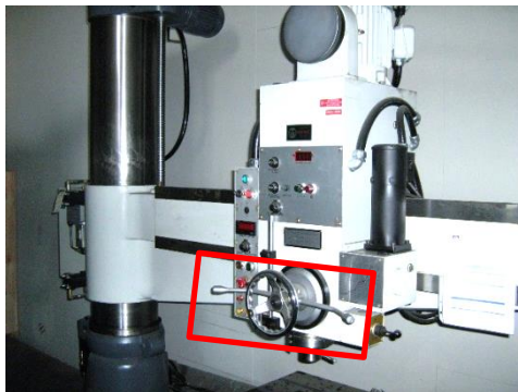
Figure 6. 2 handles situated on the guide wheel could interfere with other buttons
